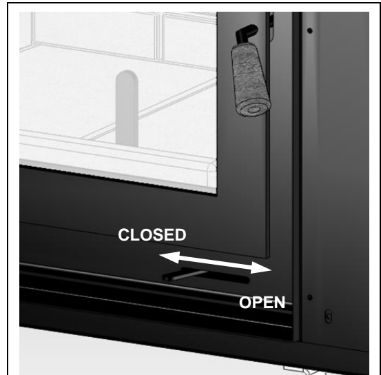
Figure 2 Combustion Air Control
